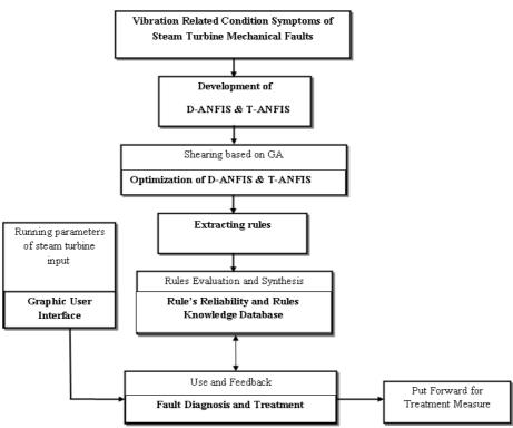
Figure 1: Flow Chart for Fault Diagnosis and Treatment
